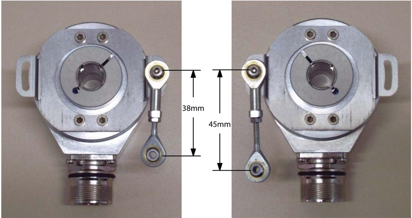
Ball joint holes are 3mm Dia. the dimensions are the same for AROD-2.5, the AROD-M4 distance between the two mounting holes is 40mm to 48mm. The rod should be as close as practical to parallel with the centre axis
