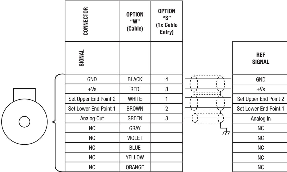
\* Note: Overall shield required; twisted pair cable not required, pairs shown only for convenience
