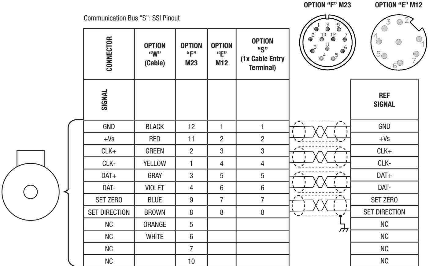
\* NOTE: Twisted pair cable required with overall shield; individual pair shielding recommended. Obey pairing as shown
