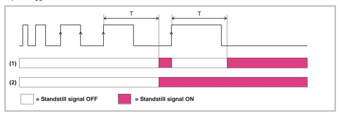
In order to get a standstill signal at all, the time distance between two positive edges must become greater than the setting "T".
